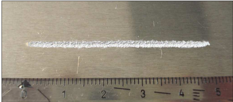
Fig.5: Aluminium plate erosion test
